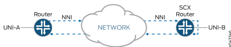
Figure 51: Testing End-to-End Service in Ethernet Loopback Mode
