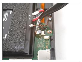
• Use a pair of tweezers to pull the right Joy-Con sensor rail's cable straight out of its connector on the motherboard.
