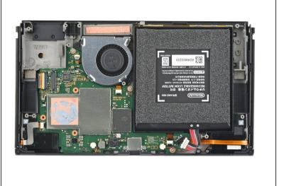
• Use a Phillips driver to remove the three 3 mm screws securing the fan to the frame.
