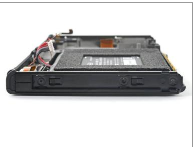
• Use a Phillips driver to remove the 3.8 mm screw securing the left Joy-Con sensor rail to the frame.
