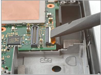
• Use an opening tool, spudger, or your fingernail to flip up the hinged locking flap on the display's ZIF connector.
