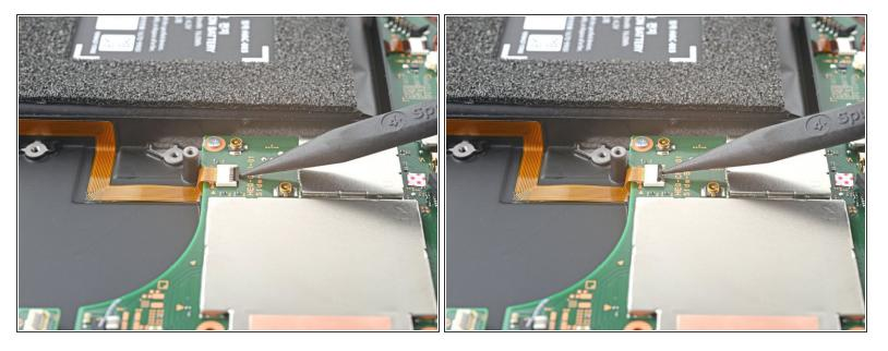
Use an opening tool, spudger, or your fingernail to flip up the small, hinged locking flap on the power button board's ZIF connector.
