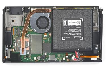
Use a Phillips driver to remove the three 3 mm screws securing the heat sink to the motherboard.
