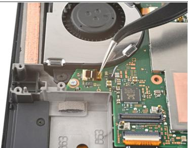
Use a pair of tweezers to pull the fan cable straight out of its connector on the motherboard.
