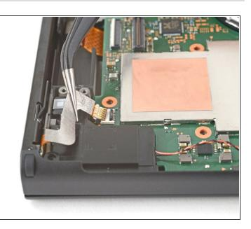
Use a pair of tweezers to pull the right Joy-Con sensor rail's cable straight out of its connector on the motherboard.
