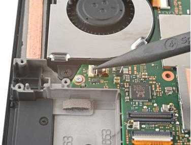
• Use the tip of a spudger, an opening tool, or your fingernail to flip up the small, hinged locking flap on the fan cable's <u>ZIF connector</u>.
