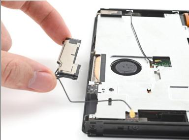
Remove the primary Wi-Fi antenna.
