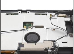
Use tweezers, or your fingers, to reroute the primary antenna's coaxial cable out of its slots in the shield plate.
