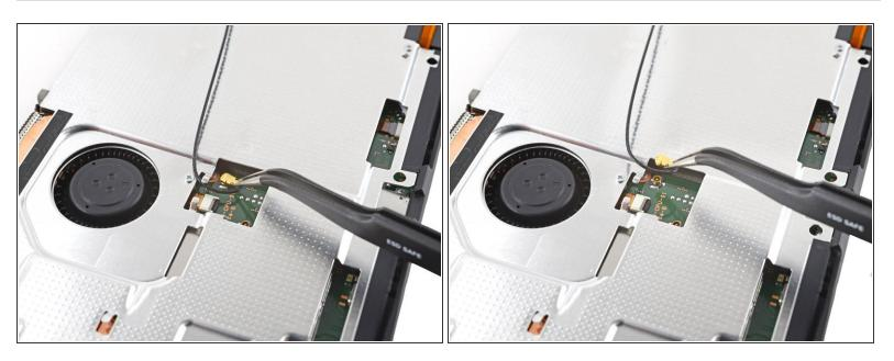
Use tweezers, or your fingers, to pull up and disconnect the secondary Wi-Fi antenna's coaxial cable.
