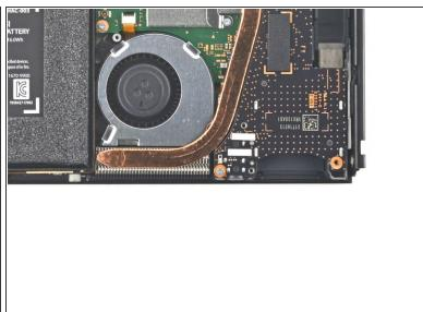
Use a Phillips driver to remove the 4 mm screw securing the daughterboard to the frame.
