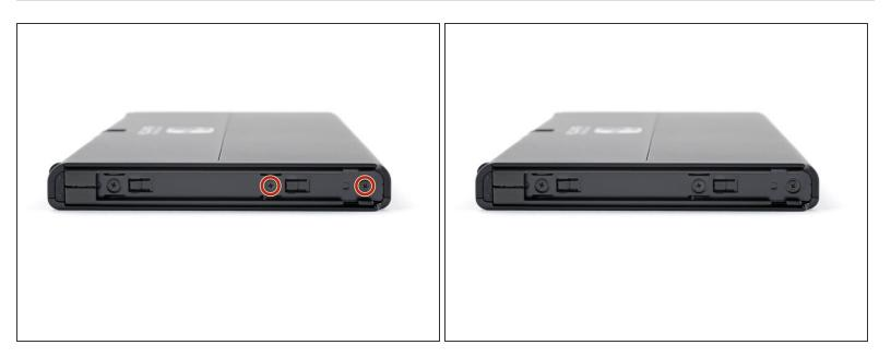
Use a Phillips driver to remove the two 3.8 mm screws securing the left Joy-Con sensor rail to the rear case.
