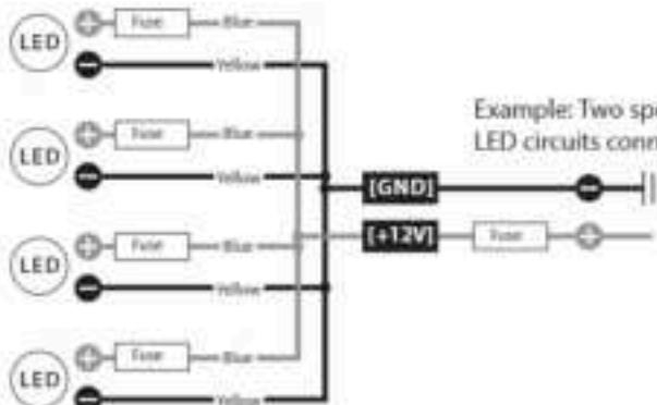
Example: Two speaker pairs of LED circuits connected in parallel.
