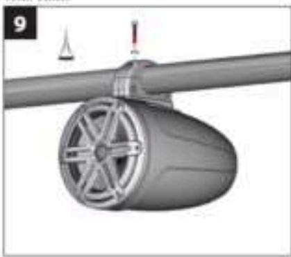
Remove one of the 1/4 - 20 x 1-1/4" Machine Screws at a time. Apply Loctite® Red Thread-Locking Compound to the screw end, reinstall, and fully tighten. Repeat the process for the other three screws.
