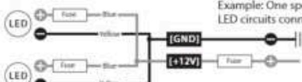
Example: One speaker pair of LED circuits connected in parallel.
