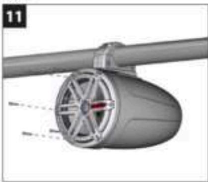
If a different speaker angle is desired, remove the #8 x 1-1/4" Pan Head Screws and #8 Flat Washers securing the speaker in the enclosure.
