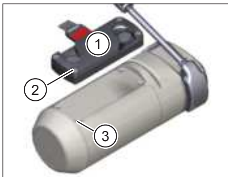
Fig. 3: Fasten FIDLOCK® Force Connector to Range Extender
