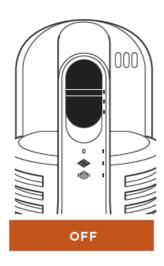
Slide switch to the top to turn off power.
