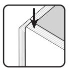
Insert tabs of Back C into the rectanglular slots on Side A, as shown.
