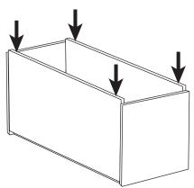
Apply force on part to secure. Parts will be flush with each other when fully locked.
