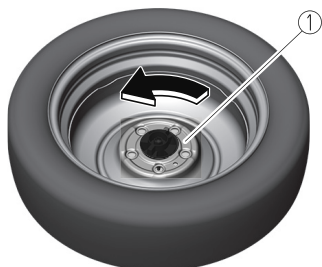
1. Spare tire hold-down bolt
