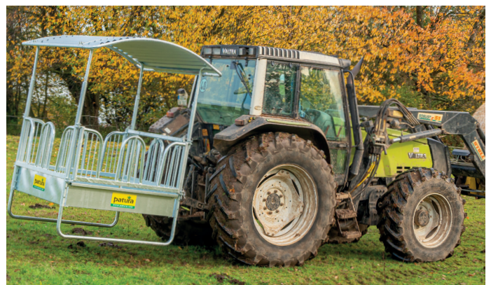
Transport using a 3-point linkage, up to 10 km/h when empty
