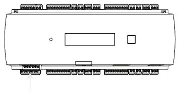
Figure 4.7: Location of the power supply connector
