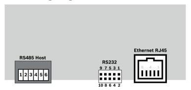
Figure 11.1: Connectors on upper PCB
