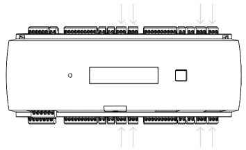
Figure 4.17: Location of the relay output connectors
