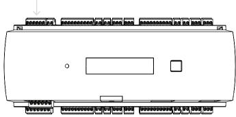
Figure 4.14: Location of the RS-485 extension module bus
