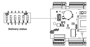
Figure 7.2: DIP switches
