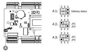
Figure 4.5: Location of ground jumper RS-485 host interface
