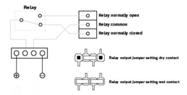
Figure 4.18: Wet mode and dry mode of the AMC2 relay outputs
