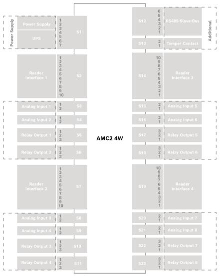
Figure 11.3: Connector blocks of the AMC2-4W
