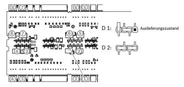
Figure 4.20: Location of the relay output jumpers (bottom side)
