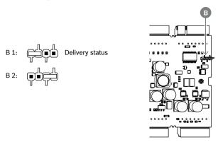
Figure 4.6: Location of ground jumper bottom side
