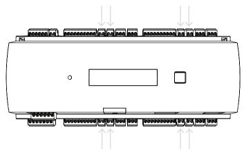
Figure 4.21: Location of the analog input connectors
