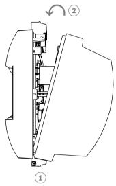
Figure 4.4: Closing the case
