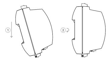
Figure 4.1: Mounting the controller on a mounting rail
