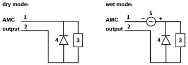
Figure 4.19: Recovery diode schematic
