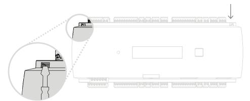
Figure 4.3: Opening the controller's case
