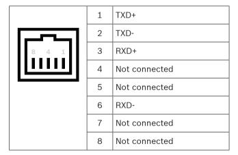
Tab. 11.5: Ethernet Network socket (RJ45)
