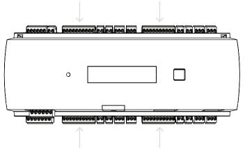
Figure 4.16: Location of the Wiegand interfaces for external devices
