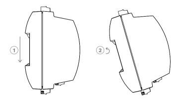
Figure 4.2: Unmounting the controller from a mounting rail
