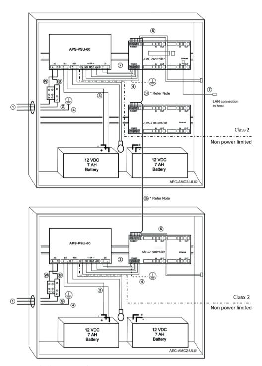
Figure 6.1: Example of mountings with extensions
