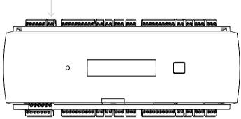
Figure 4.22: Location of the tamper protection contact
