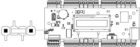
Figure 4.12: Settings for RS-485 four wire connection
