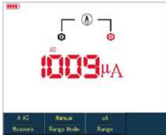
Figure 5-10 Measuring AC Current lower than 4Ma
