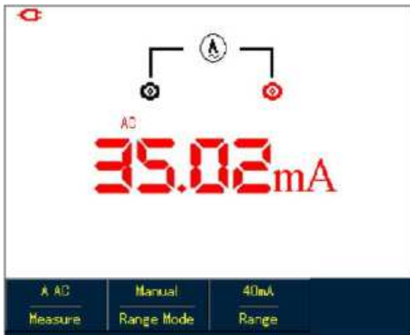
Figure 5-18 Measuring AC Current Lower than 40mA
