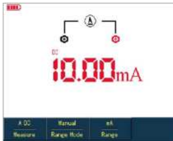
Figure 5-8 Measuring DC Current lower than 400mA
