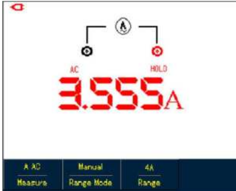
Figure 5-21 Freezing Measurement Values
