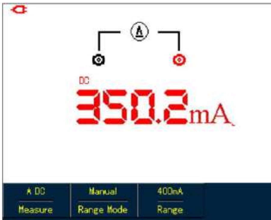
Figure 5-15 Measuring DC Current within 40mA-400mA
