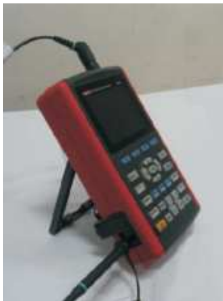
Figure 3-2 Compensation Output Connection
