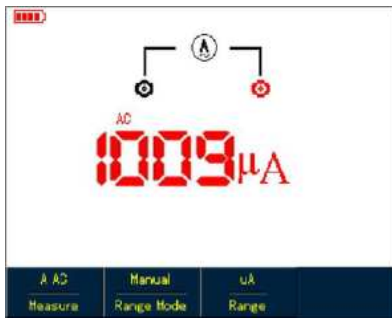
Figure 5-17 Measuring AC Current Equal to or Lower than 1mA
