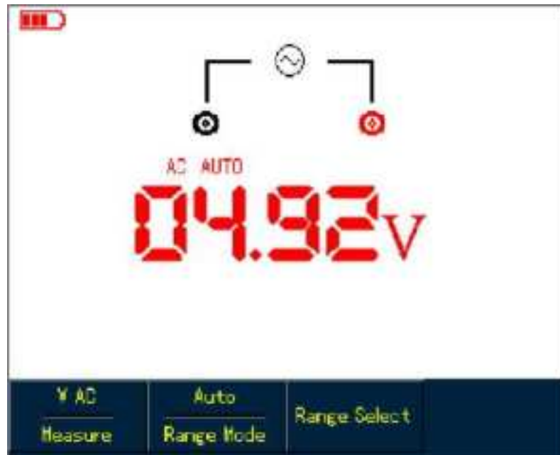
Figure 5-6 Measuring AC Voltage
