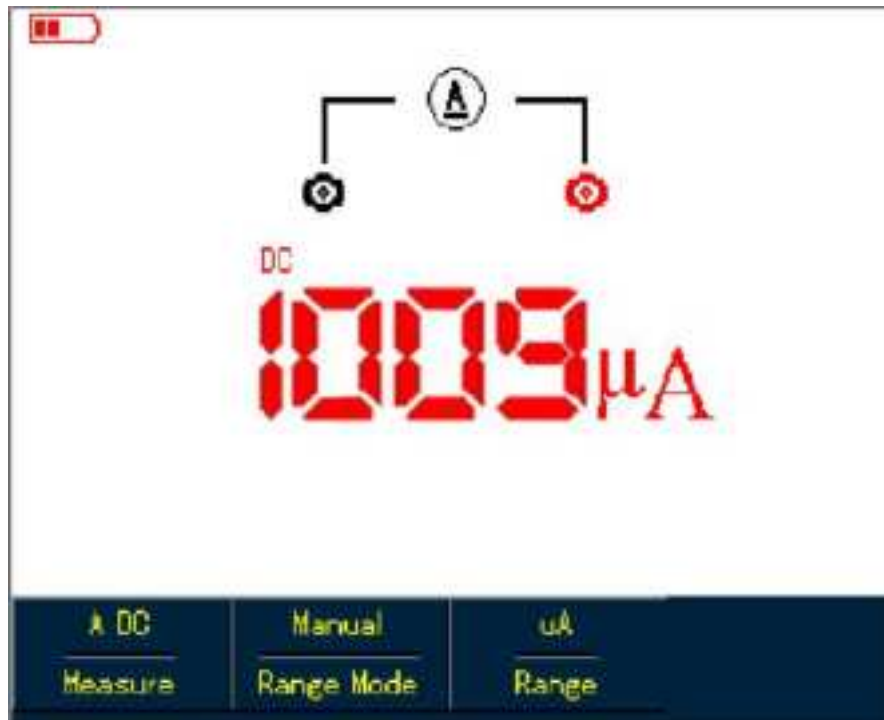
Figure 5-13 Measuring DC Current Equal to or Lower than 1mA
