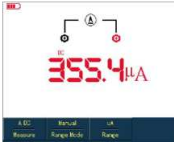
Figure 5-7 Measuring DC Current lower than 4Ma
