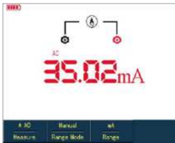
Figure 5-11 Measuring AC Current lower than 400mA
