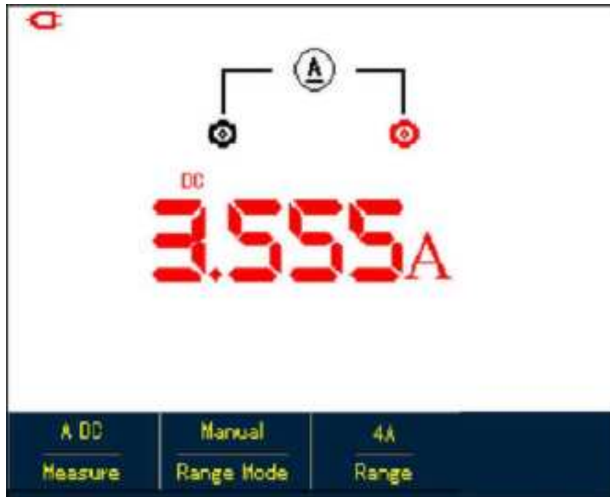
Figure 5-16 Measuring DC Current Greater than 400mA
