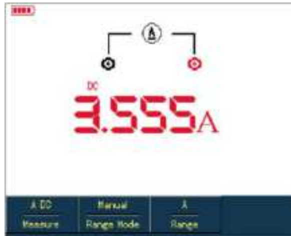
Figure 5-9 Measuring DC Current Greater Than 400mA
