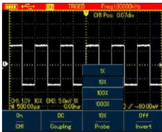
Figure 4-4 Adjusting Probe Factor
