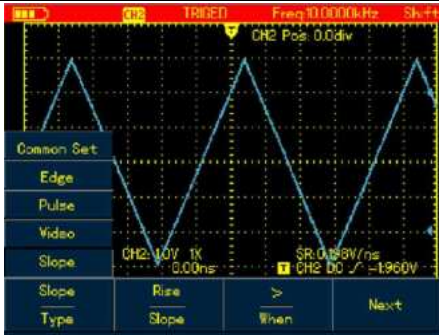
Figure 6-12 Trigger-Slope Type (Page 1)
