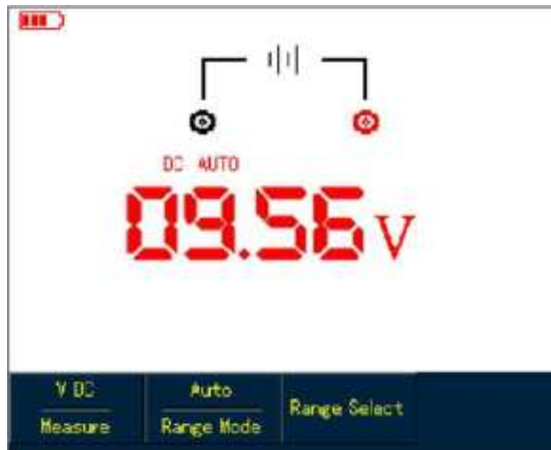
Figure 5-5 Measuring DC Voltage
