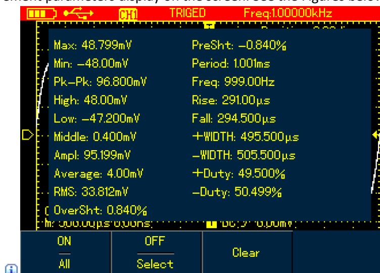
Figure 6-16A UTD1000CL measures all parameters
