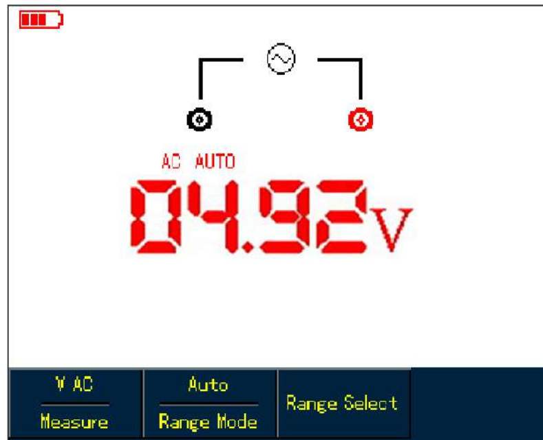
Figure 5-6 Measuring AC Voltage
