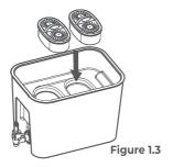
**Step 5:** Install filter into reservoir. Press firmly to ensure a tight seal. **[Figure 1.3]**
