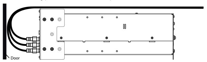
Mounting for a bigger bending radius of the connection cables (use rear holes of the brackets)
