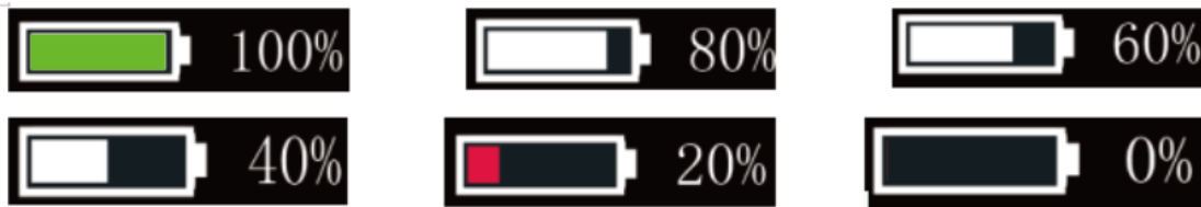
Battery SOC Indication Interface
