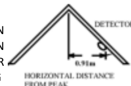
Figure 5: RECOMMENDED LOCATION TO MOUNT SMOKE DETECTORS IN ROOMS WITH SLOPED, GABLED, OR PEAKED CEILING
