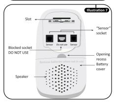
8. Press control unit holder or hanging hook firmly into slot in back of control unit (see illustration 6 and 7). 9. Place mattress firmly on top of sensor pads. If the mattress cannot be in contact with the sensor pads, or if the bed base is soft, padded or contains springs, place extra plywood on the bed base, place the sensor pads on the plywood and place the mattress firmly on top.
