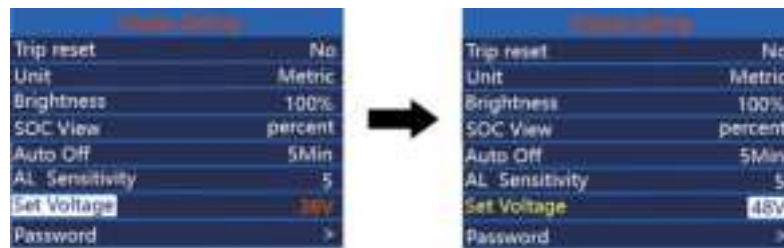
Battery voltage setting interface
