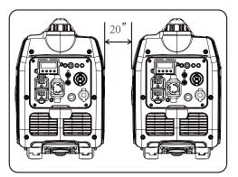
If not spaced apart, the exhaust heat from one unit may discolor or melt the plastic on the other unit.
