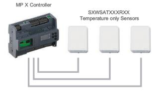
Each sensor uses an I/O port on the controller. Maximum number of inputs varies by controller type.
