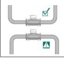
If possible, install HYDRUS 2.0 BULK at a low-lying point in a pipeline to prevent the formation of air bubbles.
