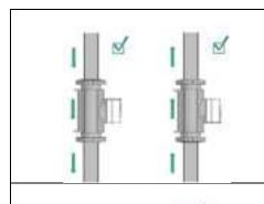
Installation in horizontal and vertical position.
