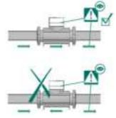
**Caution**: Check that the direction of the water flow matches the direction of the arrow located on the casing.
