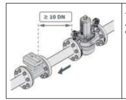
There must be no air bubbles in the measuring section. A distance of 10 pipe diameters must be maintained from devices that can generate cavitation.
