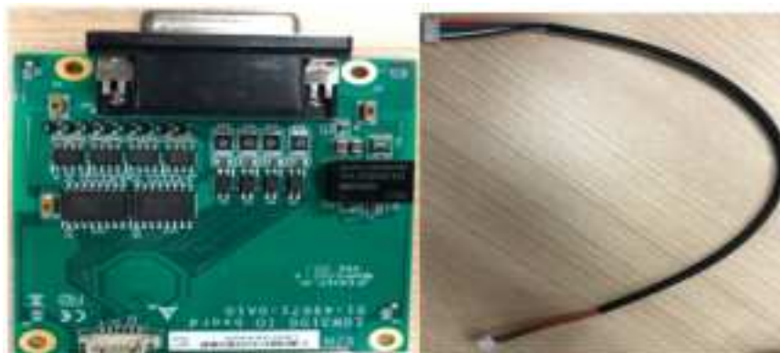
Figure 135. PCA9535 GPIO expander board and connector
