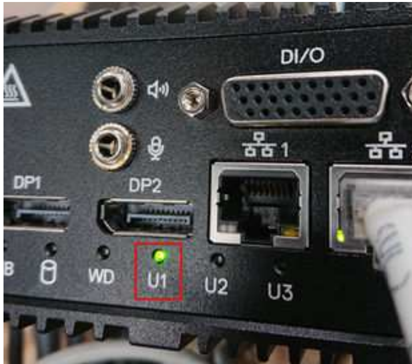
Figure 130. GPIO USER_LED illuminated
