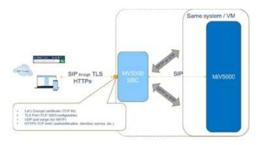
Daisy Chain configuration: The Mitel Dialer works with 2 MiVoice 5000 SBC. The first one is in DMZ, the second one is in LAN
