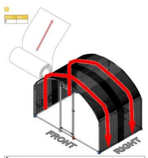
In the package you will find the poultry net. When attaching the net to the chicken run structure, do not precut the net. Instead, roll the net along the tubes and cut it. The arrows on the illustrations indicate the flow of the net. Follow the arrows to roll and cut the net. Use zip-ties to fasten the net to the tubes. There will be overlaps between the nets.
