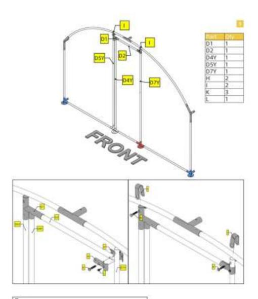
For screw L, you will need a power tool to drive it into tube 07Y.
