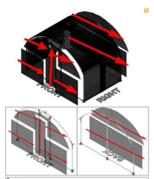
For the net placed at the back of the chicken run, we suggest rolling the net roll without measuring or precutting the net like last step. For the net placed in the front, it's easier to measure and cut the net, and then fasten the cutted net to the tubes.
