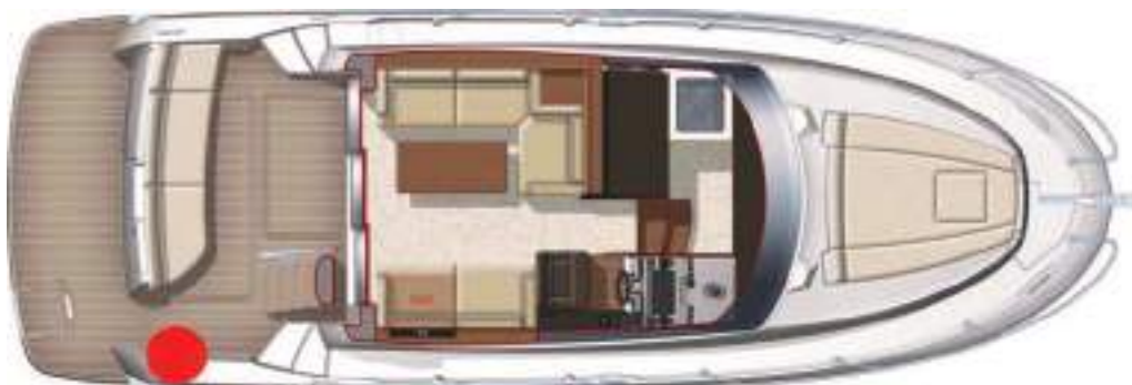
Location - Shower + Socket - Shore water
