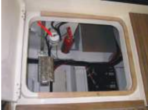
Hydraulic fluid tank - Trim
