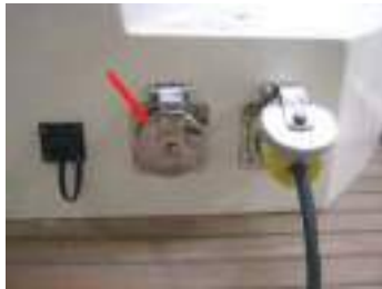
Seawater inlet (Reference 4)
