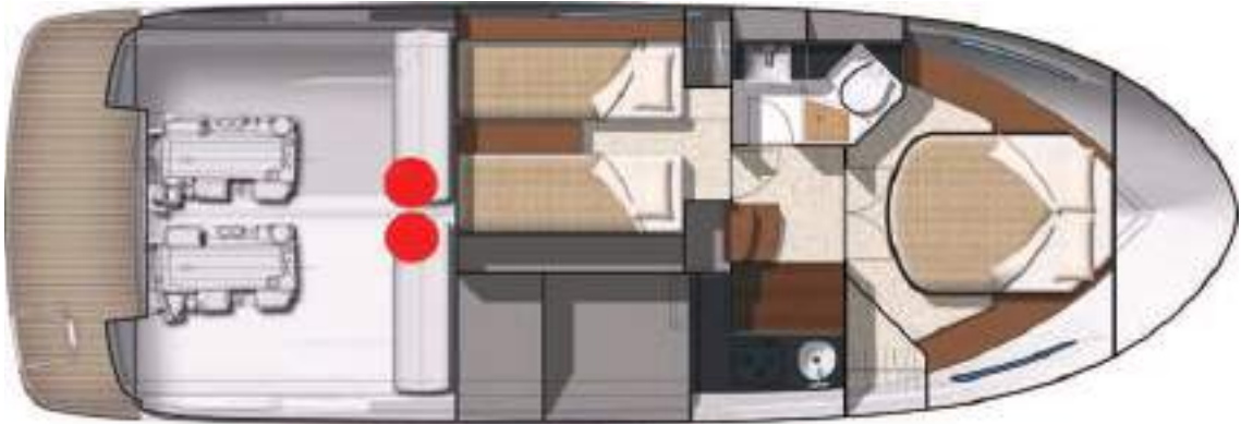
Fuel supply valve
