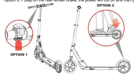
**NOTE:** As an additional safety feature, the scooter is designed to cut power to the motor when either brake option is applied.
