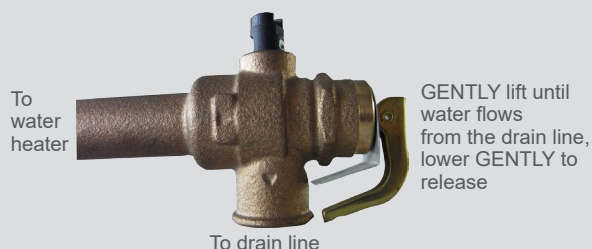
How to operate the easing gear
