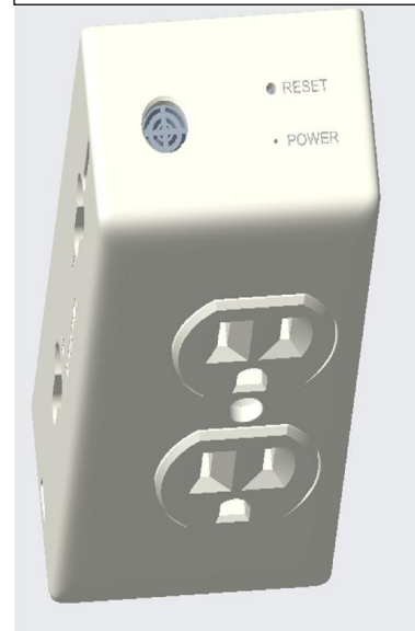
Image 22: Top view of Location Beacon AC Power
