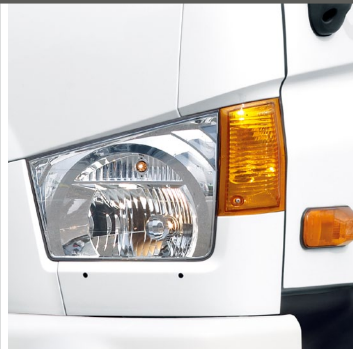
MFR Headlamps (Multi Focus Reflection)
