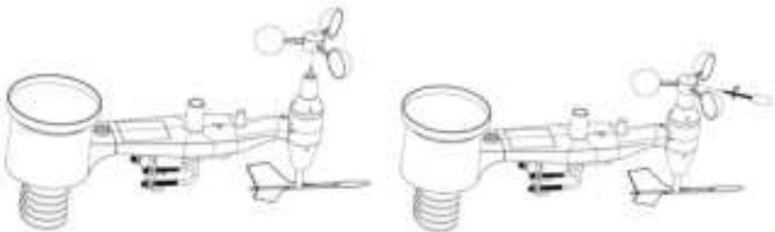
Figure 8 Wind speed cup installation diagram
