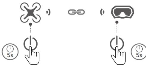
2. Press and hold the power button on the aircraft until the battery level LEDs start to blink in sequence.
