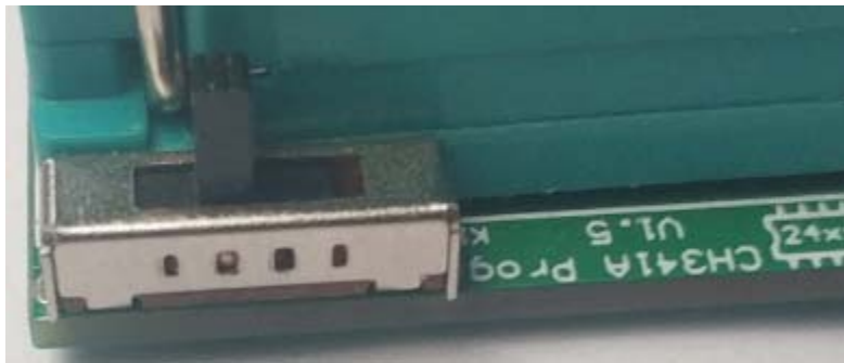
c) 3.3v toggle switch position reference (default)
