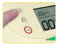
Press power button to turn on the device.
