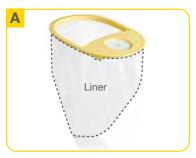
Expand liner prior to installing in warmer.
