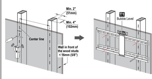
Locate your studs. Verify and mark the center of the stud by finding the stud edges using awl and stud finder. Line up the holes with your stud center line. Level the wall plate and mark the pilot hole locations.
