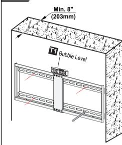
Level the wall plate and mark the pilot hole locations.
