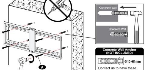
Use the hammer to knock anchors (not included) into the concrete wall. Be sure the anchors are seated flush with the concrete surface.
