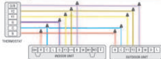
Wiring for 2H and 2C thermostat
