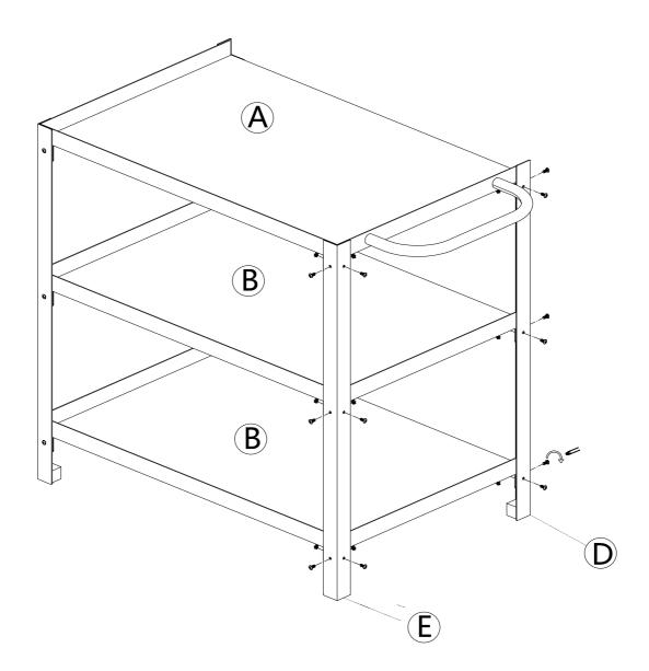
1. Assemble A, B and D, E together, and tighten screws G and H.
