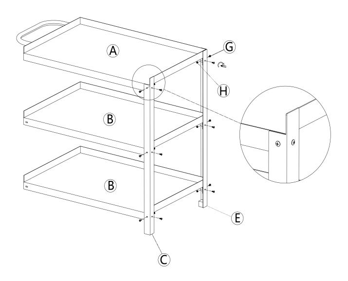
1. Assemble A, B and C, E together, and tighten screws G and H.
