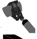
3) Slide RVibrake3 back towards the seat until RVibrake3 reaches the edge of the seat pan.
