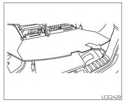
3. Carefully remove the wheel cover to avoid potential damage to the side trim.
