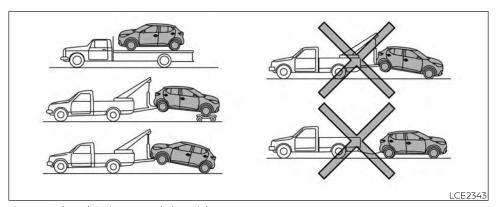
Front-Wheel Drive models with Continuously Variable Transmission (CVT)
