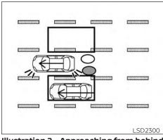
Illustration 2 - Approaching from behind Illustration 2: If the driver activates the turn signal when another vehicle is in the detection zone, then the system chimes (twice) and the side indicator light flashes.
