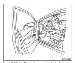
SRS Air Bag Warning Labels (located on the sun visors) SUPPLEMENTAL AIR BAG WARNING LABELS
