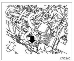
**HR16DE** engine **ENGINE SERIAL NUMBER**
