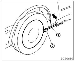
Removing wheel cover (if so equipped)
