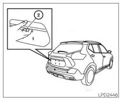
· Doors do not lock with the door handle request switch equipped) or the liftgate request switch (if so equipped) with the Intelligent Key inside the vehicle and a chime sounds to warn you. However, when an Intelligent Key is inside the vehicle, doors can be locked with another Intelligent Kev.
