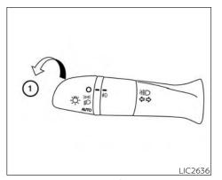
Autolight system (if so equipped) The autolight system allows the headlights to turn on and off automatically. The autolight system can:
