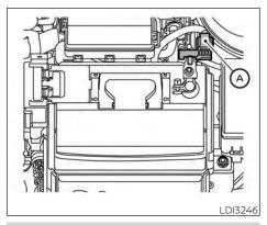
The current sensor (A) is located near the battery along the negative battery cable. If you add electrical accessories to your vehicle, be sure to ground them to a suitable body ground such as the frame or engine block area
