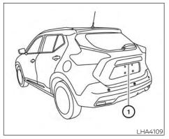
To display the rear view, the Rear View Monitor system uses a camera located just above the vehicle's license plate 1.
