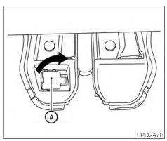
1. Move the cover (A) by using a screwdriver or a similar tool available on hand.
