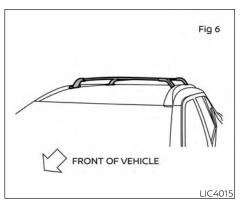
6. Tighten all 4 bolts to 8-9 N-m torque using a T-30 TORX® torque wrench.
