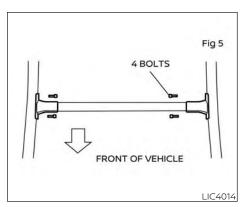
5. Make sure that the FRONT crossbar is in proper position with respect to the roof rack rail attachment positions, and loosely install all 4 bolts on FRONT crossbar using the T-30 TORX® screwdriver provided.
