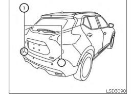
The RCTA system uses radar sensors ① installed on both sides near the rear bumper to detect an approaching vehicle.
