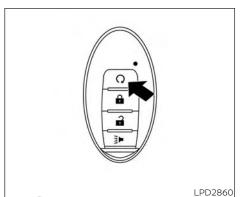
The  $\Omega$  button will be on the NISSAN Intelligent Key® if the vehicle has Remote Engine Start. This feature allows the engine to start from outside the vehicle.
