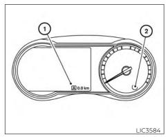
**Type A (if so equipped)**Odometer/Twin trip odometer
