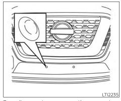
For alignment purposes, there are two marks on the bumper fascia to indicate the correct position for each screw.
