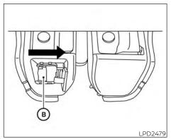
2. Then move the inside lever (B) by using a screwdriver or similar tool available on hand. The liftgate will open.
