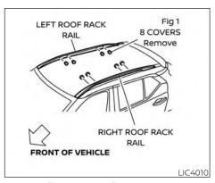
1. Manually remove all 8 protective caps from the roof rack rails. See Fig. 1.
