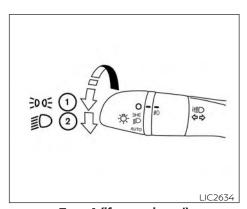
Type A (if so equipped) HEADLIGHT CONTROL SWITCH Lighting
