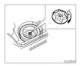
6. To loosen the bolt, turn counterclockwise.
