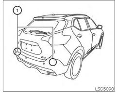
The BSW system uses radar sensors (1) installed near the rear bumper to detect other vehicles in an adjacent lane.
