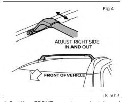
4. Position FRONT crossbar onto left and right roof rack rail; and adjust right support in and out until it fits securely into position.
