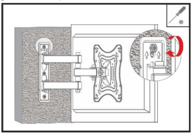
10) Attach the 2 plastic caps to protect the bracket and its screws.
