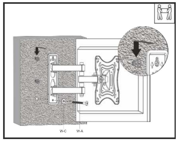
09) Tighten all 3 screws with a Phillips screwdriver.
