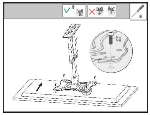
06) When using the longer M-B screws, you can also use the additional plastic rings (M-C).
