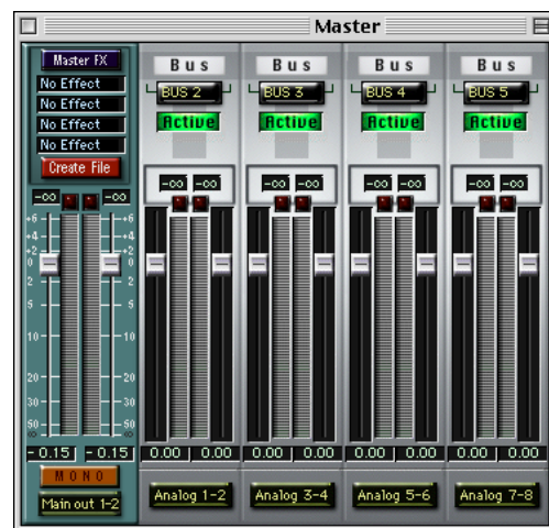
Figure 10-5: Use the output buttons at the bottom of each channel strip, including the master fader, to assign 24i outputs to busses. You can then assign channels in the Monitor window to each bus as desired.
