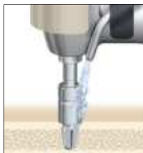
Fig.14: Drilling with Guide drill with spacer removed
