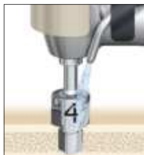
Fig.15: Drilling with widening drill
