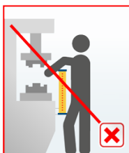
Fig. 7: Installation at a low safety distance
