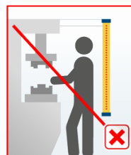
Fig. 8: At a very high safety distance, the horizontal installation of a safety light curtain is required.
