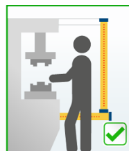
Fig. 7: Installation at a low safety distance
