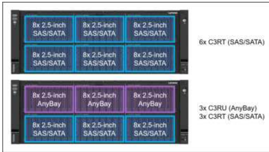
Figure 10. SR860 V4 drive bays - 2.5-inch drive bays
