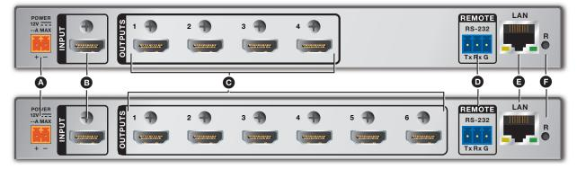
Power input — Connect the provided 12 VDC, 3.0 A power supply to this 2-pole 3.5 mm captive screw port (see the power Attention and diagram to wire the connector on page 2).
