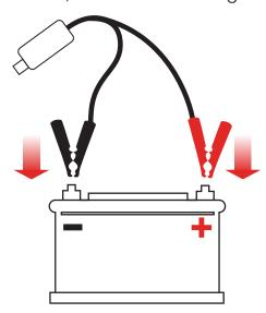
Wait for the green LED on the jumper cable to light up and then start your vehicle
