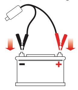
Connect the jumper cables to the Jump Starter 1000A
