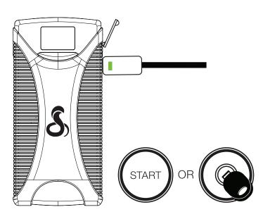
Disconnect the jumper cable from the Jump Starter 1000A and then from the battery
