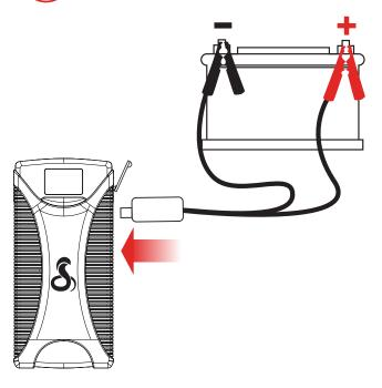
Disconnect the jumper cable from the Jump Starter 1000A and then from the battery
