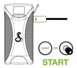
Connect the jumper cable to the Jump Starter 1000A
