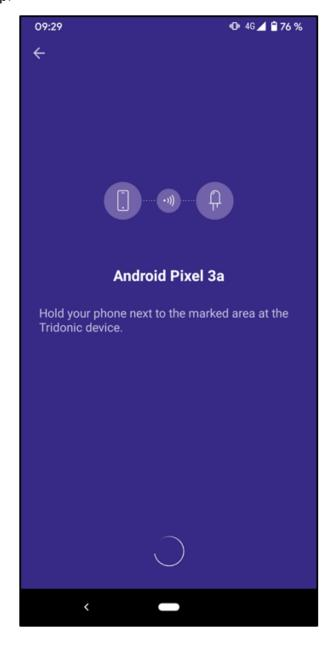
Now hold your phone or the NFC reader next to the marked area on the driver. The phone will vibrate when a connection is established. Wait for a few seconds until the driver has been read-out successfully.
