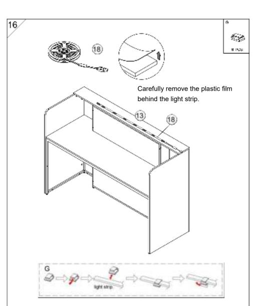
Note that G can be installed or not according to personal needs. G is used for the stick-off configuration of the light strip.
