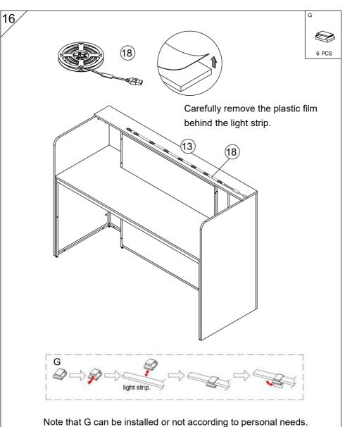
Note that G can be installed or not according to personal needs. G is used for the stick-off configuration of the light strip.
