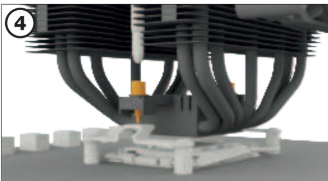
Place the cooler onto the CPU unit. Then screw the mounting bridge alternately tight. You can use the cross-tip screwdriver for this.
