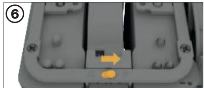
Dark Rock Pro 5 has a Quiet (Q) and a Performance (P) mode. The mode affects the maximum fan speeds and the operating noise. To change modes, first remove the magnetic top cover. Move the switch to switch between the modes.
