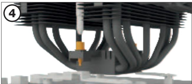
Place the cooler onto the CPU unit. Then screw the mounting bridge alternately tight. You can use the cross-tip screwdriver for this.
