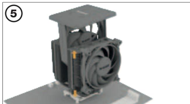
Center the Silent Wings 135mm fan from above. Then slide it into the recess between the heatsinks and press it firmly. Connect both fans via the Y-cable. You can remove the fan clips of the Silent Wings 4 120mm and adjust the height.
