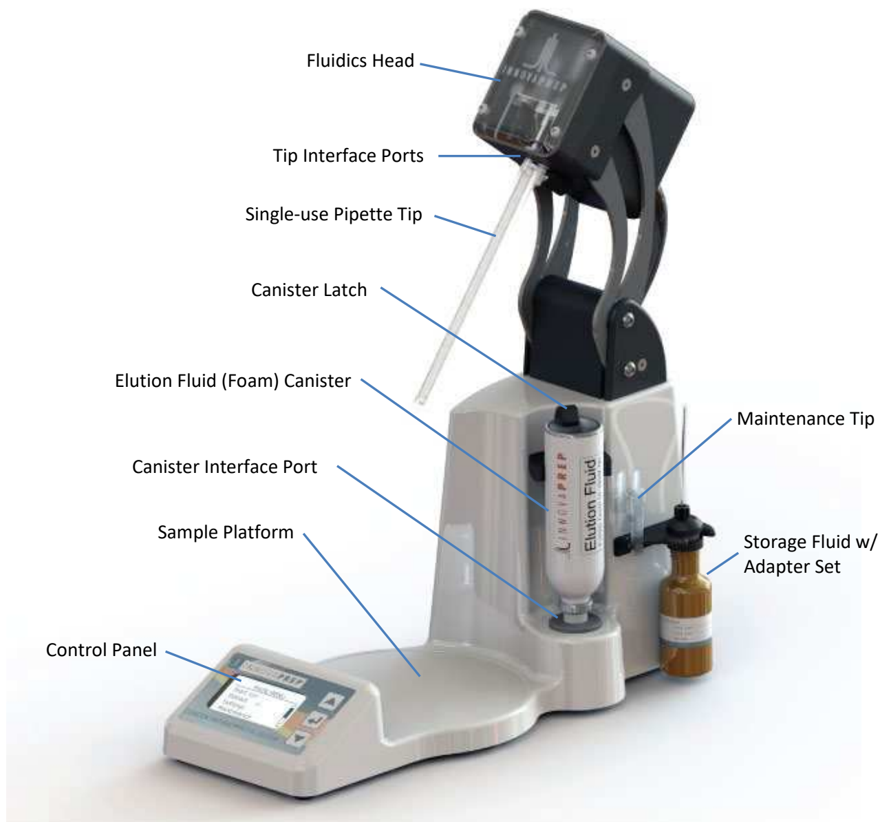
FIGURE 3.1 CONCENTRATING PIPETTE COMPONENTS - RIGHT SIDE
