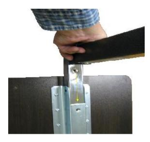
4. Align the holes in the column with the holes in the bracket on the table top. Insert and tighten the two pan head screws.
