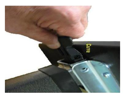
6. Make sure the trip lever sits on top of the trip rod in the column.
