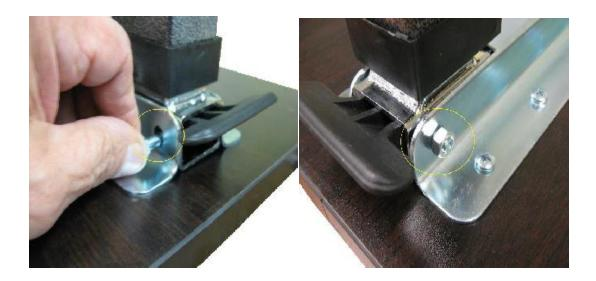
9. Place the two bolt sleeves in the base.
