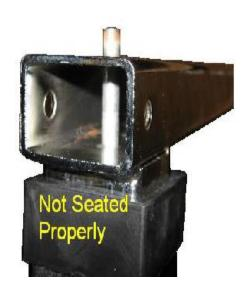
3. Hold the trip rod in place and insert the column into the bracket on the table top.
