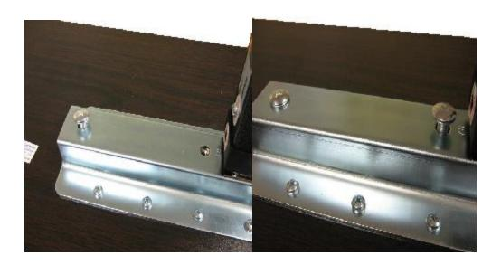
5. Insert the trip lever with the curved side facing towards the bottom of the table.
